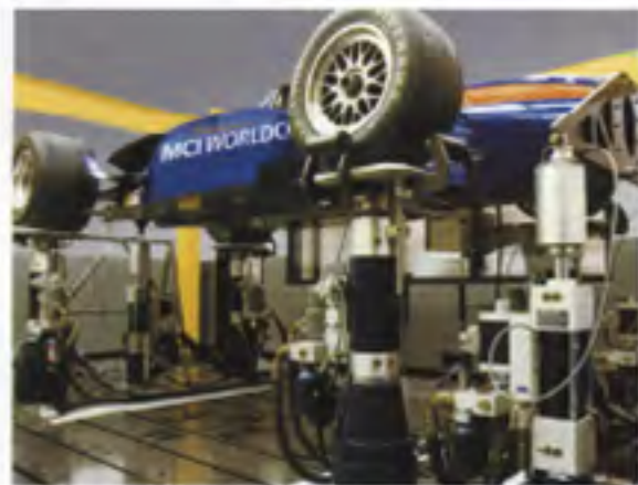
PPIM's Road Dynamics Simulator allows the team to do additional research and development in-house. The machine simulates the conditions of any track we race on, using accrued data, and tests various performance components of the car.
